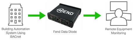
Fend supports Modbus, BACnet, and other communication protocols.
