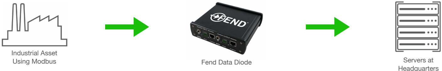
**Example 2: Connect remote equipment to your network, even when it's off the beaten path. Fend's data diodes can send sensor data over an LTE connection to your company's servers.**
