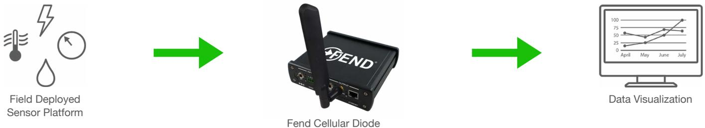
**Example 3: Listen to industrial control system network traffic and send relevant data to on- or off-premise servers for storage or analysis. Help prioritize maintenance tasks and equipment upgrades.**
